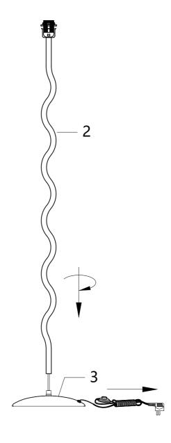
Pull out the supply cord a bit, then screw the part 2 and Base 3.
