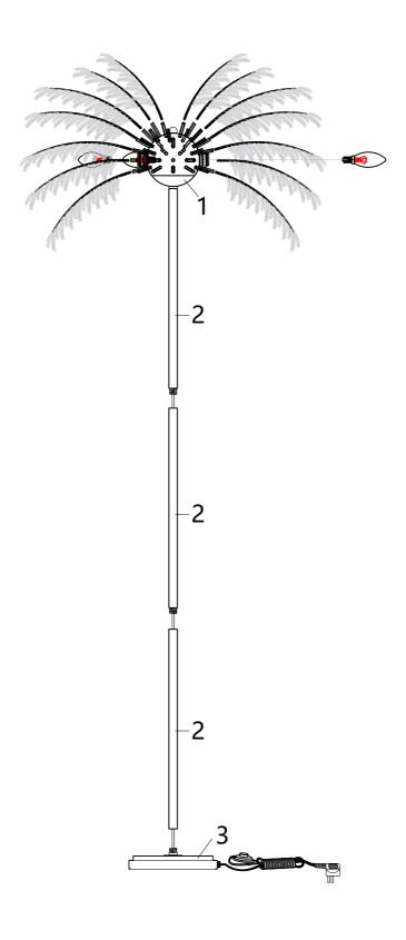
Screw 1 and 2 first, then screw between parts 2.
