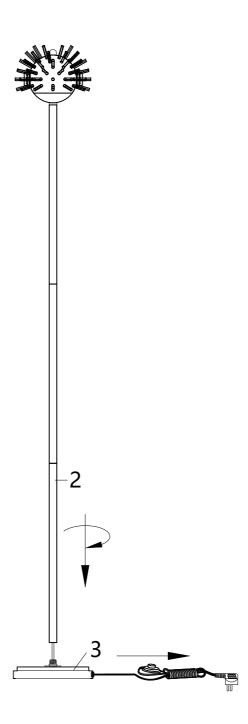
Pull out the supply cord a bit, then screw the part 2 and Base 3.
