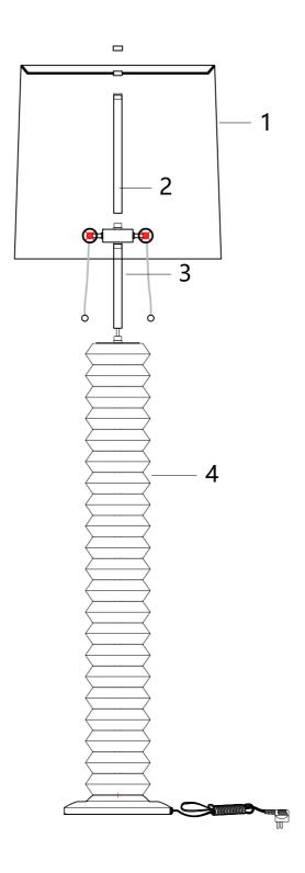
Pull out the supply cord a bit, screw the part 3 and Body 4, then fasten the 2 on the 3.
