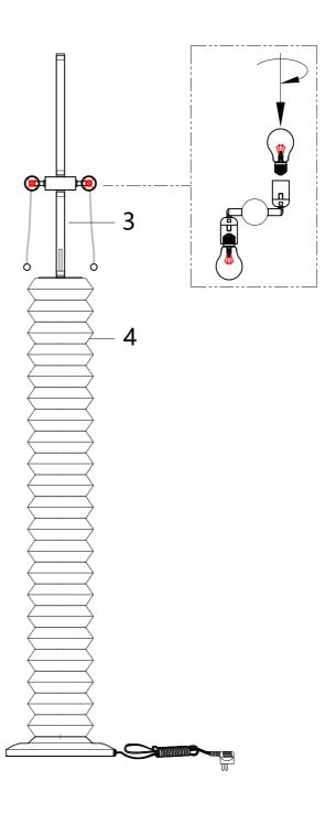
Twist out the metal nut on the 2, install the shade, then tighten the metal nut back.
