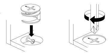
Turn cam lock clockwise to tighten.
