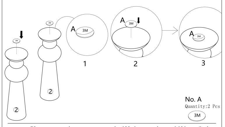
STEP 2 Please note the uneven ground will impact the stability of the product, suggest have the product on the even ground and press the glass to glue with the base strongly.
