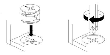
Turn cam lock clockwise to tighten.
