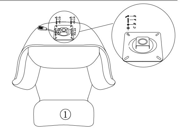
NO.A Quantity:4Pcs Screw M6\*20mm | No.B Quantity:4Pcs Lock Washer M6 | No.C Quantity:4Pcs Flat Washer M6x16mm | No.D Quantity:1Pc Allen Key M6
