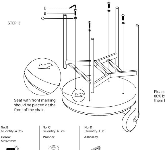
Please fasten the screws 80% by hand then tighten them fully by Allen key.
