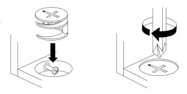
Turn cam lock clockwise to tighten.
