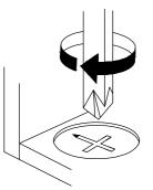
Turn cam lock clockwise to tighten.
