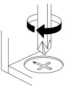
Turn cam lock clockwise to tighten.
