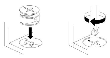
Turn cam lock clockwise to tighten.
