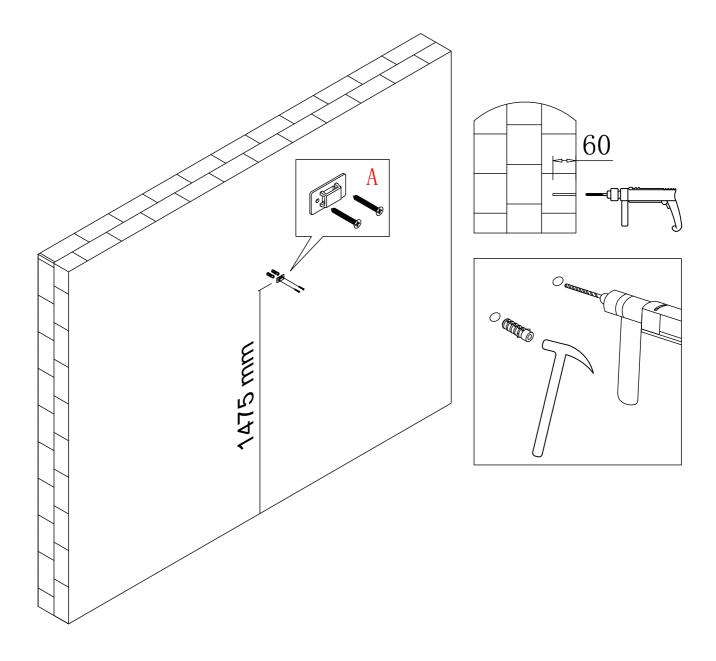
No. A Quantity:1 Sets Anti-falling Parts
