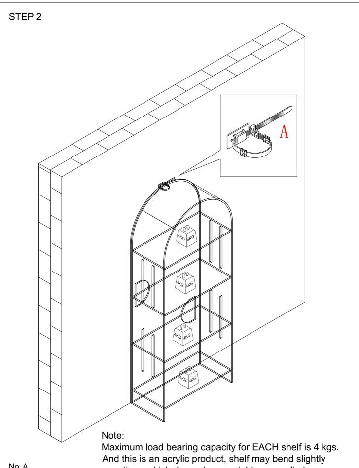
No. A Quantity:1 Sets Anti-falling Parts over time, which depends on weight you applied.
