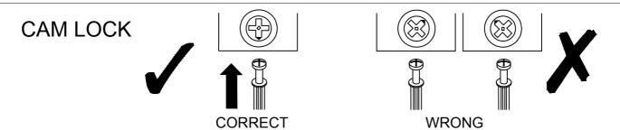
When fitting cam lock, ensure starting position is correct before you insert connecting quickfit.
