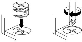
Turn cam lock clockwise to tighten.
