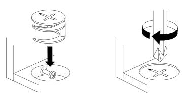
Turn cam lock clockwise to tighten.
