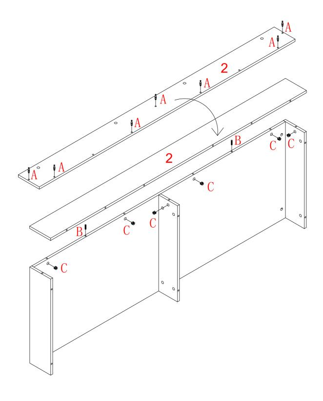
No. A Quantity:7 Pcs Cam Lock Dowel 8\*28mm No. B Quantity:2 Pcs Dowel 8\*30mm
