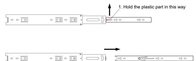
2. Pull out the inner slider for drawer box fixing
