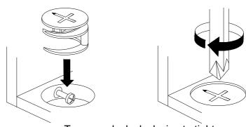
Turn cam lock clockwise to tighten.
