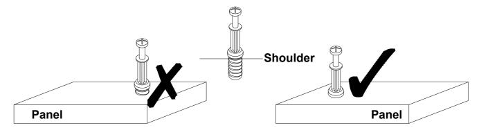
Tighten quickfit until shoulder is flush with panel. Do not overtighten or undertighten.
