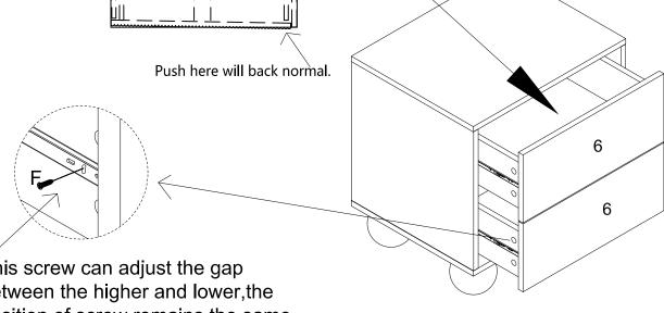
This screw can adjust the gap between the higher and lower,the position of screw remains the same, just loosen the slide rail up and down.
