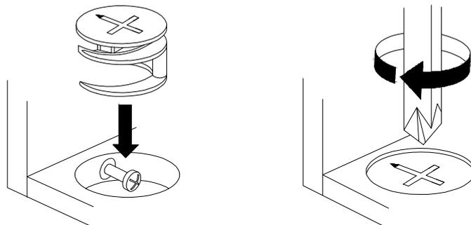
Turn cam lock clockwise to tighten.
