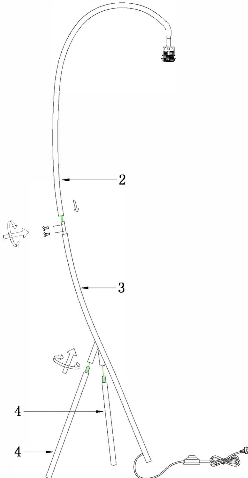
Pull out a bit of the supply cord, fasten the 4 on the tube 3.
