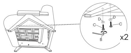
Please fasten the screws 20% by hand then tighten them fully by allen key in this step.
