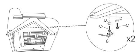
Please fasten the screws 20% by hand then tighten them fully by allen key in this step.
