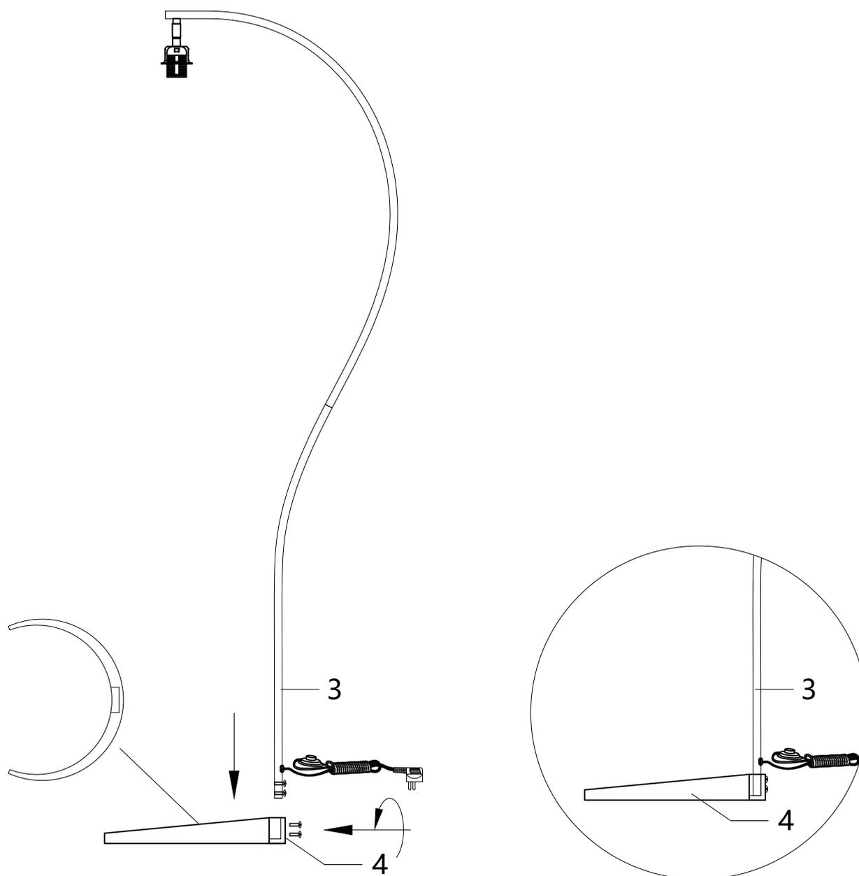
Unscrew the screws on the end of the 3, then insert the part 3 into the base 4, fasten by the screws.
