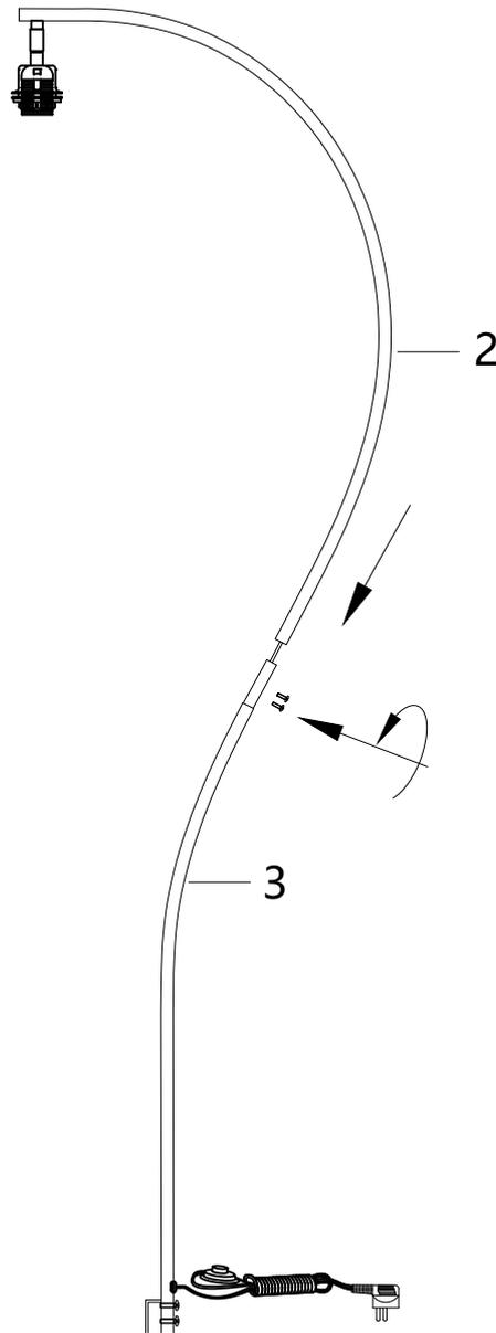
Pull out the supply cord a bit, unscrew the screws on the 3, then insert the part 2 into the 3, fasten by the screws.
